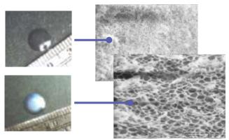
Cambridge Polymer Group performed root-cause analysis on samples provided by the client. Through an extensive and complex testing procedure staining, drying, deformation and direct microstructure visualization using SEM, the cause of the cloudiness was traced to a poorly controlled reaction process resulting in microcavitation within the lens during the swelling process as the lens hydrated.
